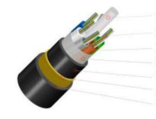
FRP Strength member Optical Fiber Loose Tube Water-blocking Tube Inner Sheath Aramid Yarn Outer Sheath
